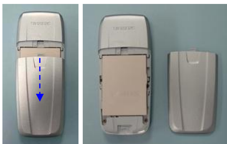
Remove Battery cover.
