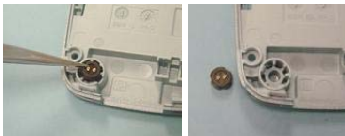
Remove Microphone
